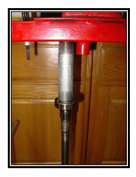
Using a hydraulic press, press the inner bearing into the shaft from the inner race so no stress is put into the balls or outer race.
