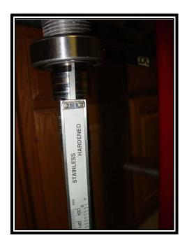
Press the inner bearing until the OEM recommended measurement of 0.91" is achieved. This will ensure a proper setback of the prop. Too much clearance will space the prop away from the veins and too little will not allow the prop to rotate when installed.
