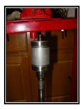
Once again press the outer bearing from the inner race into the shaft until it makes light contact with the spacers. Make sure that this does not alter the 0.91" clearance measurements required during the installation of the inner bearing
