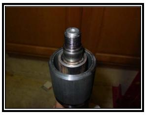
Yamaha uses an outer bearing race support that not only spaces the inner and outer bearings accordingly but it also prevents the outer bearing from being pushed in towards the seals, the nut prevents the entire shaft and prop from moving forward also. GroupK developed an inner bearing race support that minimizes the stress being put on the inner races. For those pushing those big ponies, this is a must!!!!
